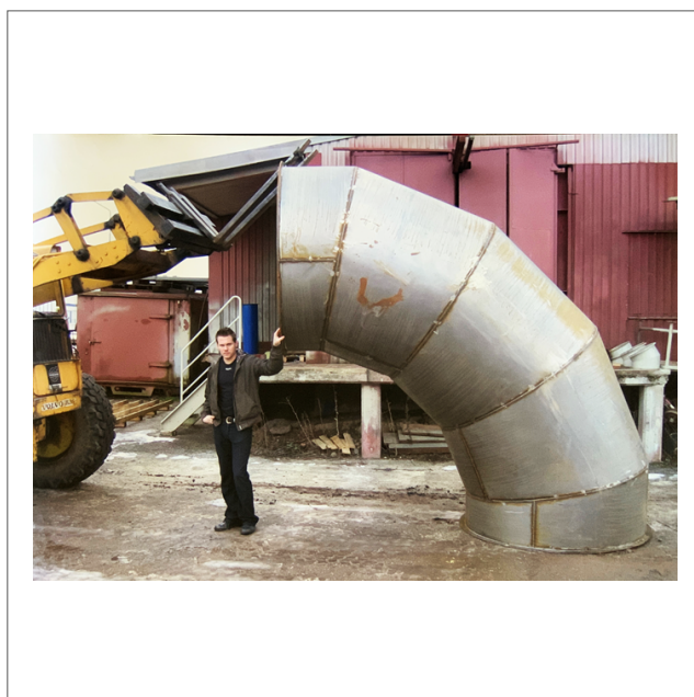
Bends with larger radius: Picture shows 2 mm black plate \varnothing 1600 mm with flange
